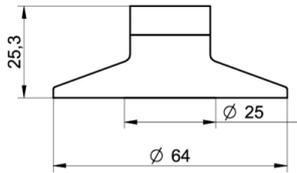
Tri-Clamp Ø 64.0, membrane Ø 25 mm (BCID: C05)
