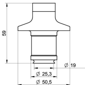
BHC 3A DN 38, membrane Ø 25 mm (BCID: B01)
