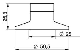
Tri-Clamp Ø 50.5, membrane Ø 25 mm (BCID: C04)
