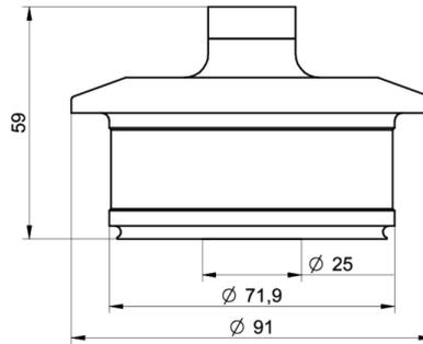
BHC 3A DN 76, membrane Ø 25 mm (BCID: B02)
