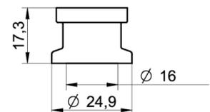
Tri-Clamp Ø 24.9, membrane Ø 16 mm (BCID: C01)
