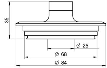
Varivent® DN 32 ... 125; 1 1/2" ... 6" (Type N), Ø 68, membrane Ø 25 mm (BCID: V02)
